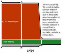
This diagram represents inefficiencies in CPU usage. Treat it as a pipe with an output flow equal to the "pipe efficiency" ratio: (Actual Instructions Retired)/(Maximum Possible Instruction Retired). If there are pipeline stalls decreasing the pipe efficiency, the pipe shape gets more narrow.
